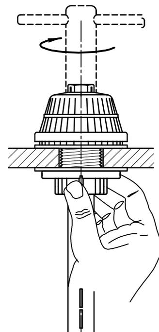
1. Nozzles have to be stored free from frost, do not install at temperatures below 0° C!
