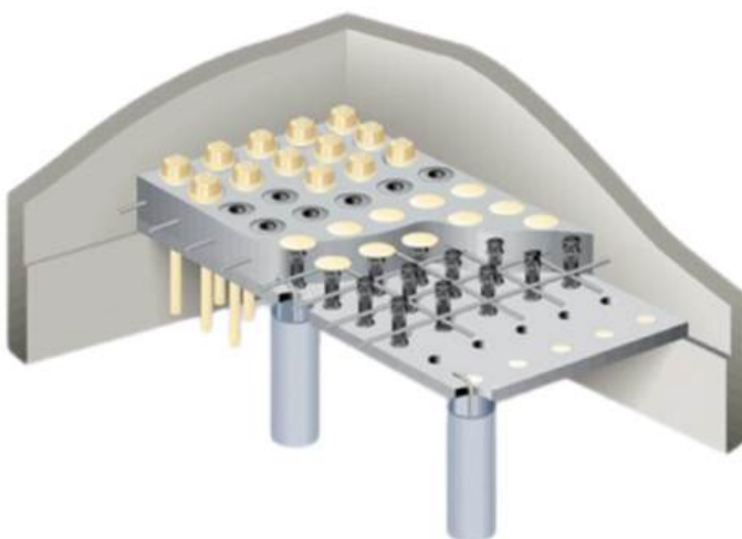
monolithic flat panel filter floor
